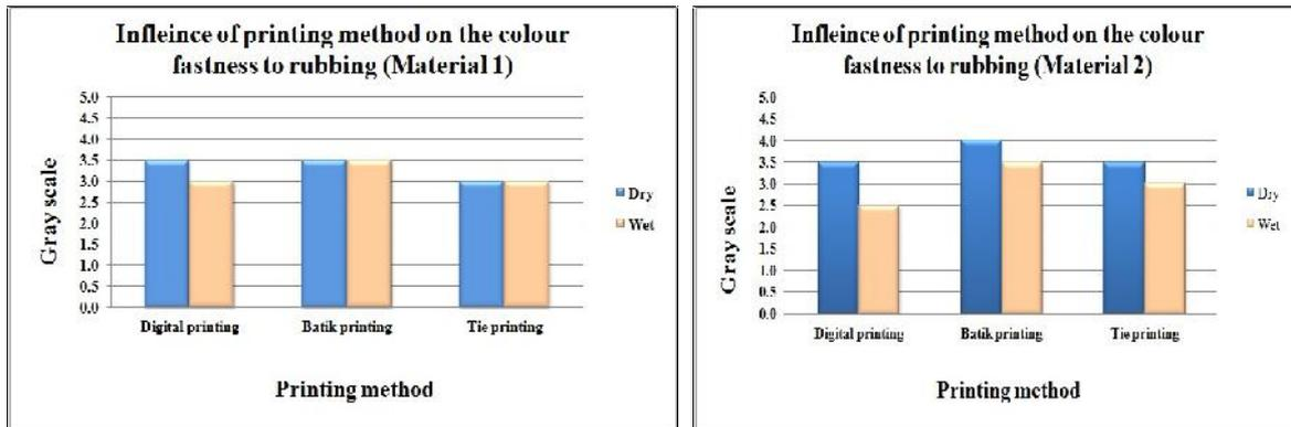
**Figure 7: Influence of Printing Methods on the Colour Fastness to Rubbing**
